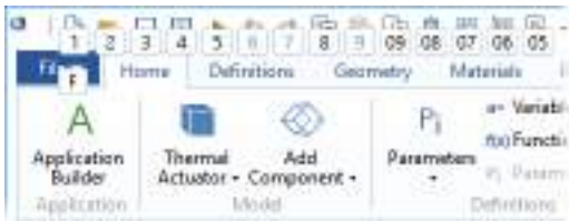
Figure 2-11: Pressing the Alt key displays the keyboard shortcuts for the Quick Access Toolbar.
