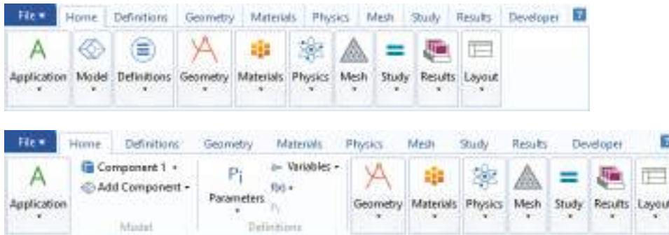
Figure 2-2: When the COMSOL Desktop is resized, the ribbon toolbar buttons are grouped together with the ribbon tab group name. In this example for the Home toolbar, all the buttons are available from a menu, such as Definitions, Geometry, Material, Physics, and so forth (top). As the window is widened, the menus expand accordingly (bottom).
