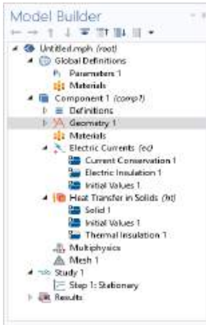
Figure 2-16: After clicking Done, a 3D Component with Electric Currents, Heat Transfer in Solids interfaces, and a Stationary study is added to the Model Builder.
